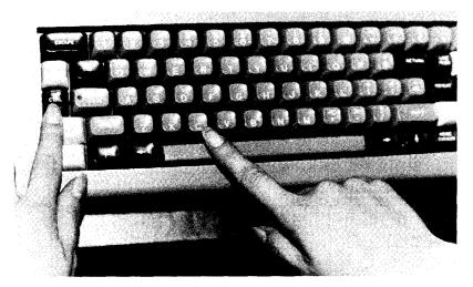
Figure 1.13: Control C Causes a Warm Boot
